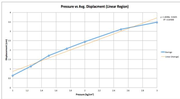
Figure III: McKibben Pressure vs Displacement
