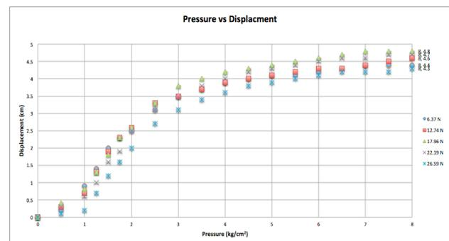
Figure II: McKibben Pressure vs Displacement Characteristic Plot
