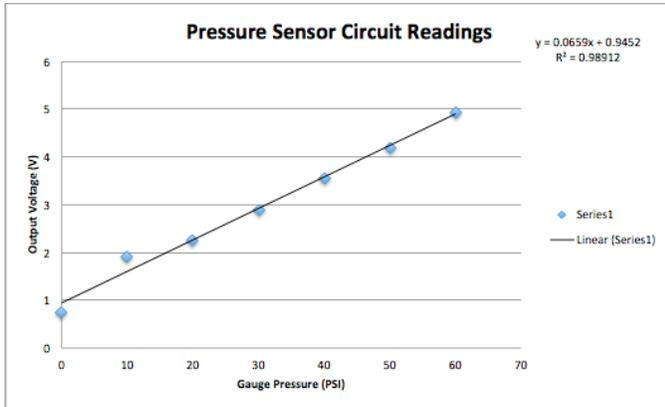
Figure I: Output Voltage of Pressure Sensor Circuit
