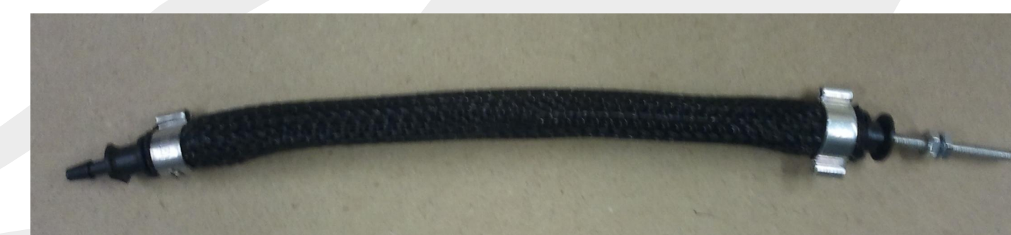
A Gaylord-McKibben Pneumatic Linear Actuator
